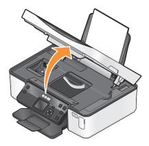
**Note:** The printhead moves to the cartridge installation position.
